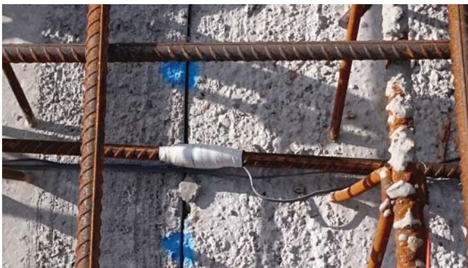
Figure 5. ER strain gauges on stitching bar across joint in planks
