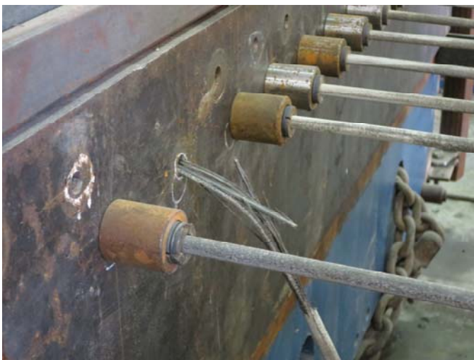
Figure 8. Tensile failure of one BFRP rebar broken after tensioning.
