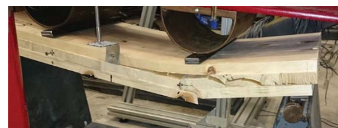
Figure 26. Rolling shear failure of Irish CLT panel
