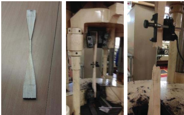
Figure 7: Tensile Test of a Tapered 700mm x 70mm x 10mm Test Pieces
