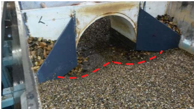
Figure 3: Scour hole for 40 l/s with 22.5° wing walls (2 mm d_{50} sediment).
