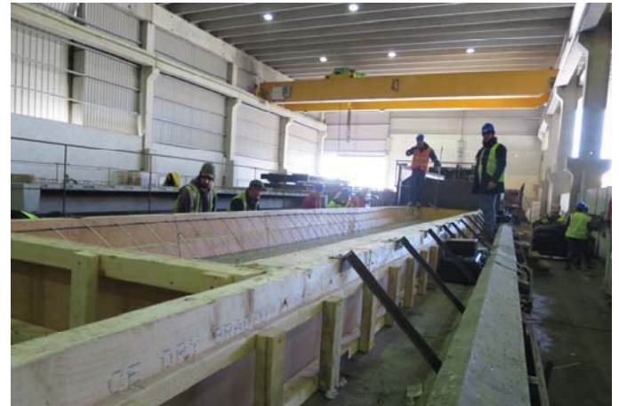
Figure 9. Positioning of shear resisting trusses in correspondence of the ribs.
