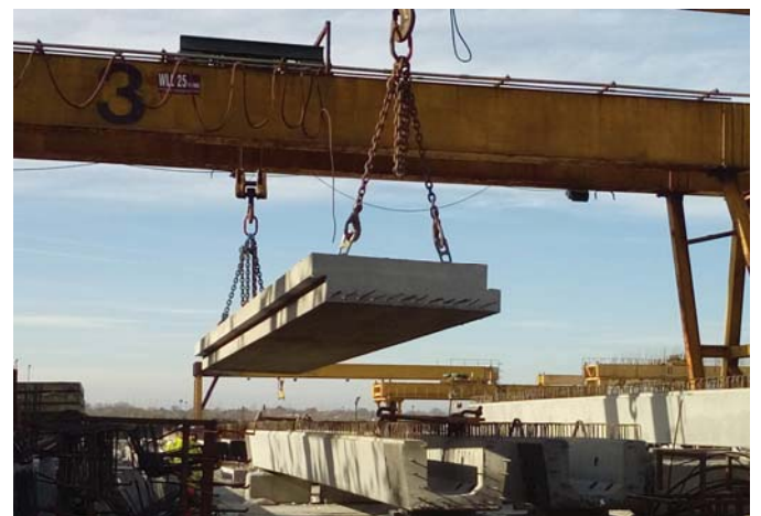
Figure 10. Steel-free pre-stressed beam moving to test rig.
