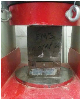
Figure 3: Cube in compression testing machine at 28 days
