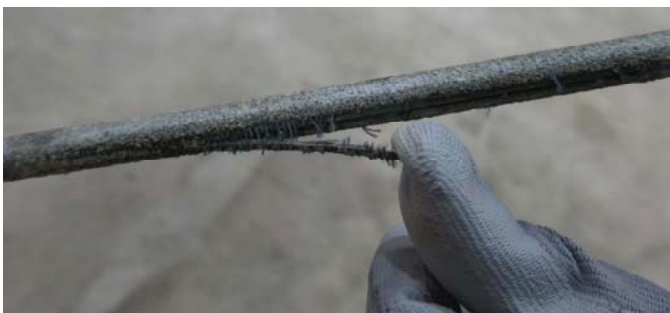
Figure 7. Particular of a BFRP rebar broken after tensioning.
