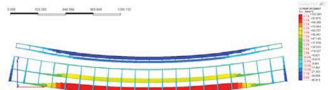
Figure 8. Output from midasFEA model displaying the stress in the reinforcement during the application of the 250kN loading for TB1-1.
