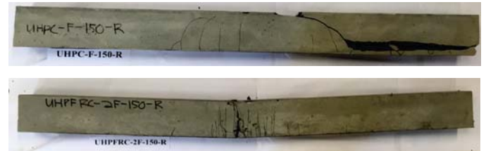
Figure 6. Failure patterns for beams (a) UHPC-F-150-R failed in shear and (b) UHPFRC-2F-150-R failed in flexure.
