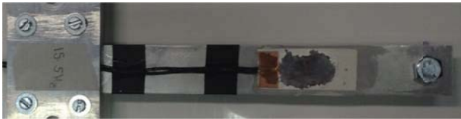
Figure 2. Experimental cantilever energy harvester with aluminium substrate and bonded PVDF energy harvester
