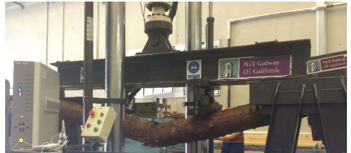
Figure 1: Four point bending test setup
