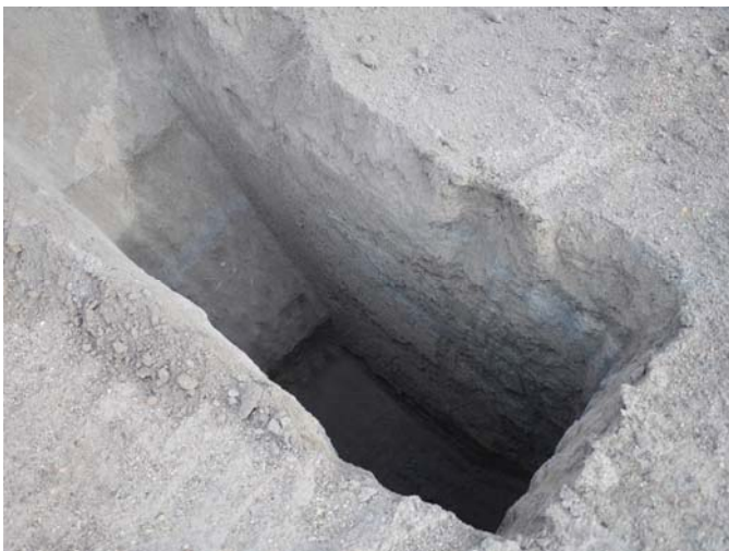
Figure 2. Image of trial pit to 2.5m in Ash Storage Area. Stability of sides shows the effect of observed weak cementation between particles.
