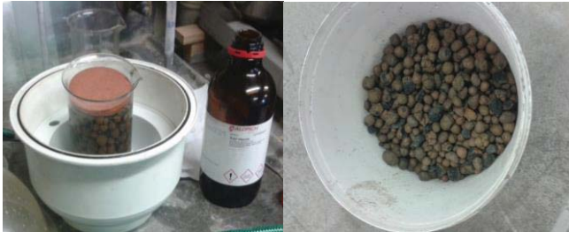
Figure 3. Manufacture of the aggregate/PCM composite
