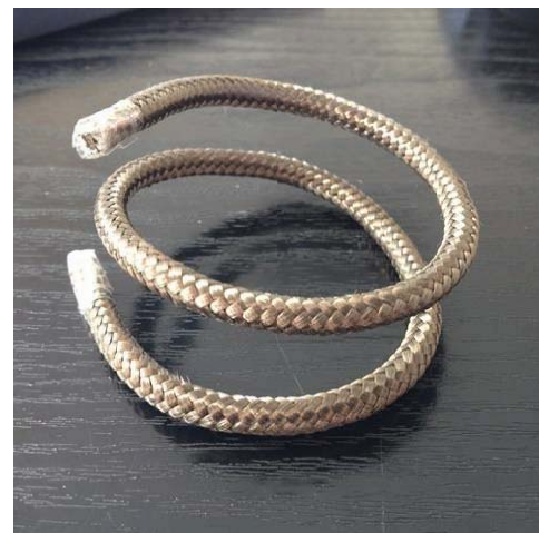
Figure 8. Braided BFRP rebar preform sample.
