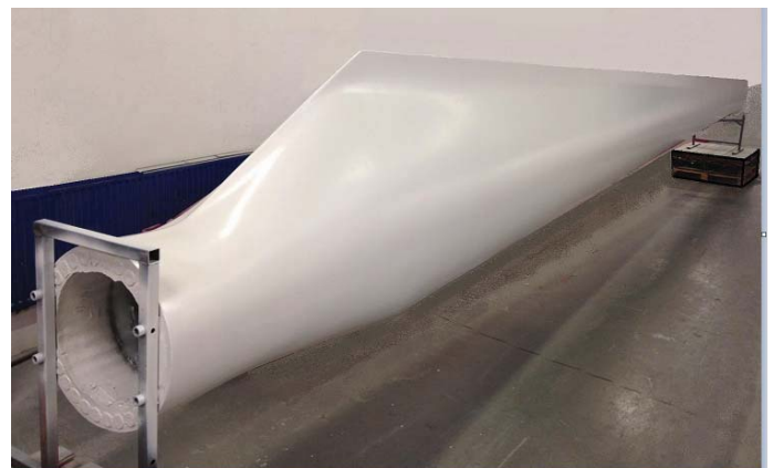
Figure 5 Commercial 13m long blade manufactured using a one-shot OOA process.
