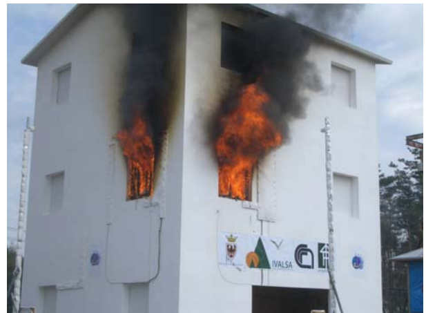
Figure 10. Fire test on 3-storey CLT building [24]
