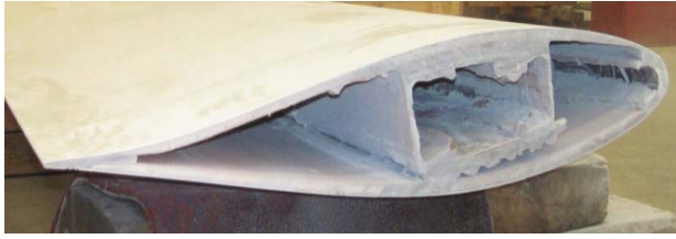
Figure 3 Section of Vestas V-27 blade showing the misalignment of central box structure with a large area of the lower spar not connected to the shell of the blade.
