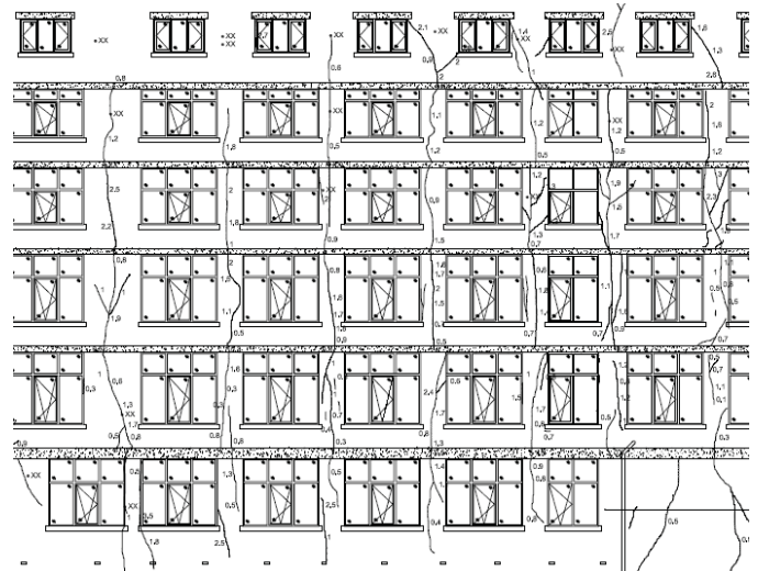
Figure 3. Section from a Visual Survey Drawing of an Early 1900s Office Building in Belfast [7]. Note Majority of Cracking between Windows with Structural Steelwork Behind.
