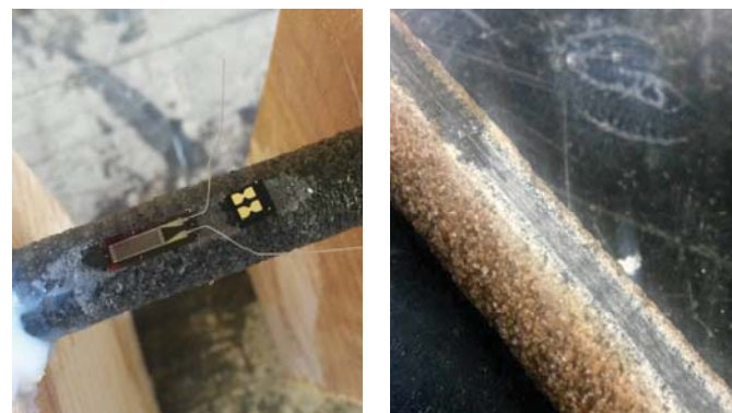
Figure 2. a) ERS gauge, b) DTG fibre mounted on BFRP rod
