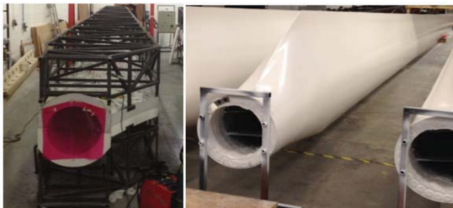
Figure 1 (Left) Integrally heated ceramic mold. (Right) 13m GF powder epoxy wind turbine blade [1].
