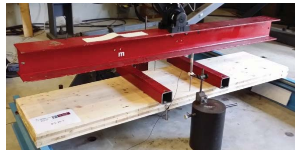
Figure 25. Out-of-plane bending test on Irish CLT panel
