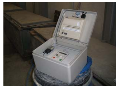
Fig. 1- Apparatus of maturity used at Banagher Precast Concrete
