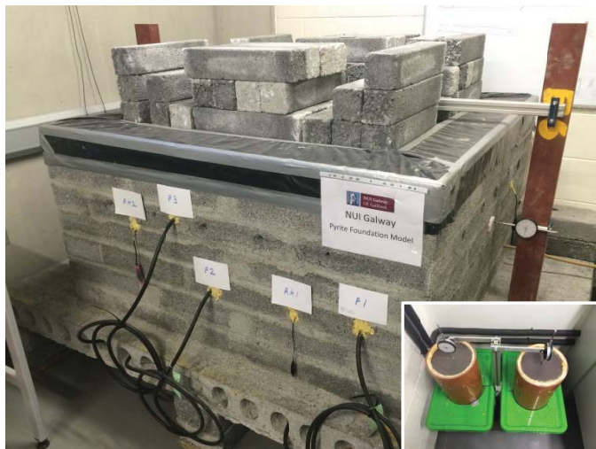
Figure 1. NUI Galway Pyrite Foundation Model, including imposed load of 3.4 kPa (inset: pipe experiments D2 and D3).
