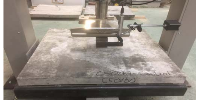
Figure 4. Slab punching load test setup.
