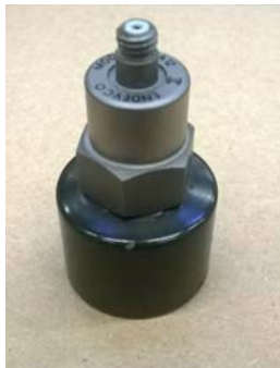
Figure 11. ENDEVCO 752A12 accelerometer with a magnet base.
