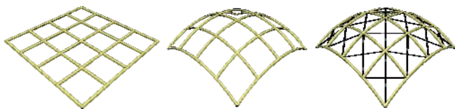
Figure 1: From a flat grid to a lattice shell to a gridshell
