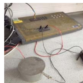
Figure 2 Bulk resistivity test equipment and sample
