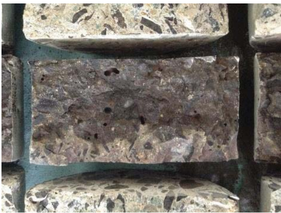
Figure 10 Splitted sample slices sprayed with Silver Nitrate
