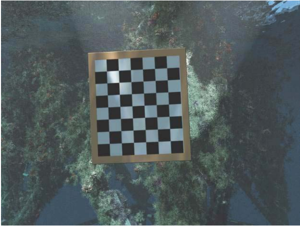
Figure 5. Checkerboard calibration for the virtual scene.
