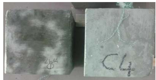
Figure 5. Leakage of PCM from the lightweight aggregate
