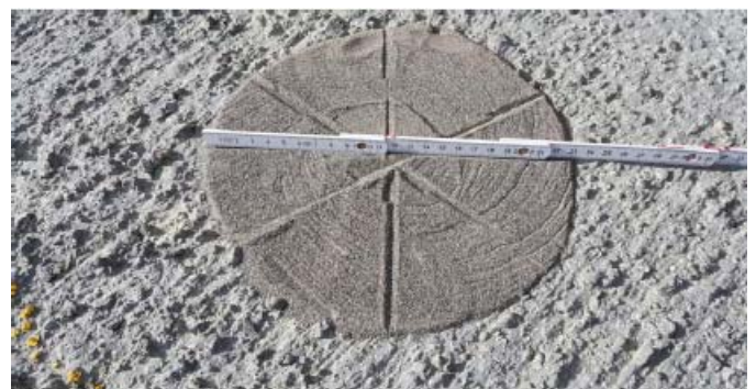
Figure 6. Sand spread into circular fashion over rough surface. (Source - Banagher Precast Concrete).
