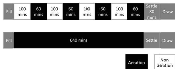
Figure 2: Operation of conventional SBR versus IASBR
