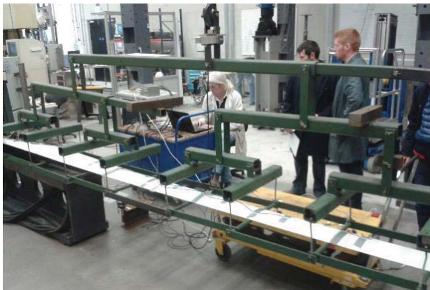
Figure 1. Whiffle tree rig applies the total load to the blade at eight locations distributed along its length.
