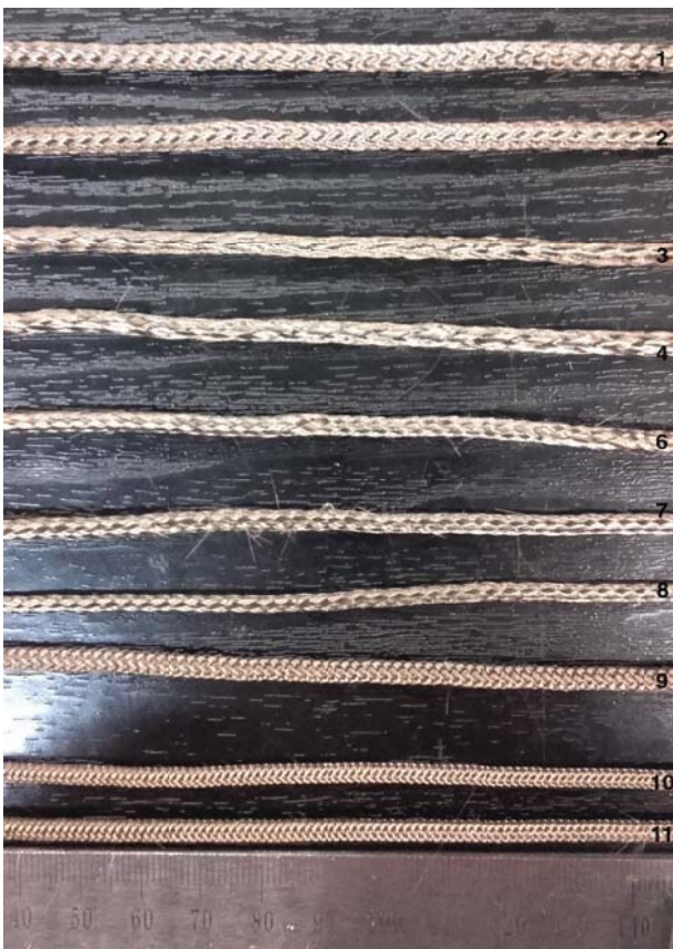
Figure 6. Braided core production trials.
