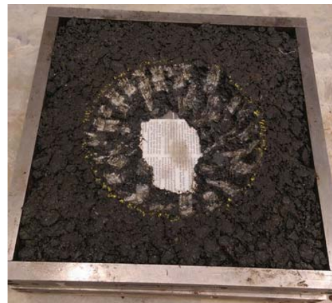
Figure 1. A simulated pothole for geopolymer repair material investigation.
