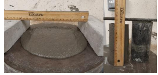
Figure 3. Flow table and cylindrical slump test to determine fresh properties of mortar.
