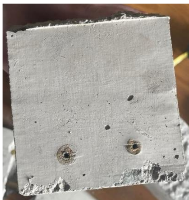
Figure 13: End of beam after tensile failure showing negligible movement of the reinforcement into the beam
