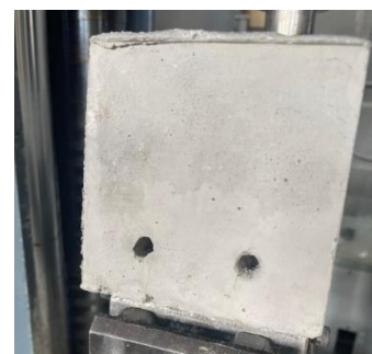
Figure 10: End of beam after bond failure showing inward movement of bamboo reinforcement into the beam
