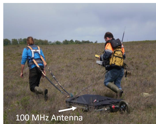
Figure 37. Man-hauling 100 MHz GPR antenna across an upland peat area (Picture shows Andy Trafford iCrag / UCD and Ian Sharkey APEX Geophysics)
