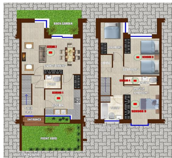
Figure 2. Drawing indicating the locations of the five sensors provided in each typical house.
