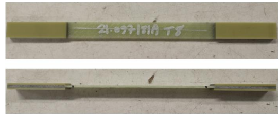
Figure 6. Cut and Tabbed Test Coupon
