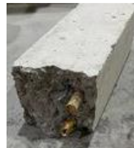
Figure 9: Half of an unnotched reinforced beam displaying tensile failure in the culms
