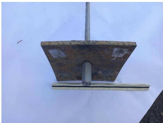
Figure 18. Deformed Anchor 14 following exhumation
