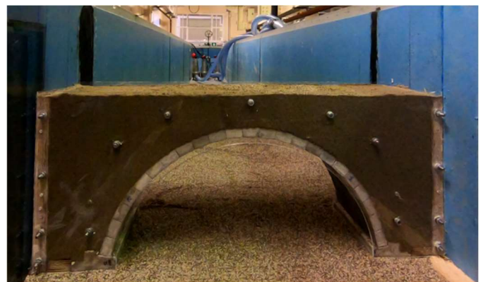
Figure 2. 1:10 scale FlexiArch model on the sediment bed.
