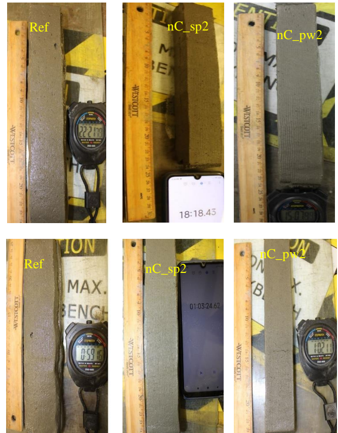
Figure 9. Printing component of 'Ref', 'nC_sp2' and 'nC_pw2' mixes at 15 minutes and 60 minutes respectively.
