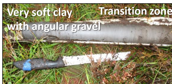
Figure 29. Jowsey peat auger and image of base of borehole showing transition between peat and underlying mineral soils
