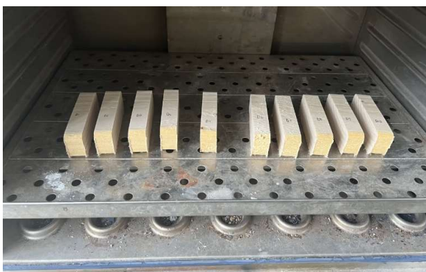
Figure 6. Oven drying method used to determine moisture content of timber before manufacture of CLT panels
