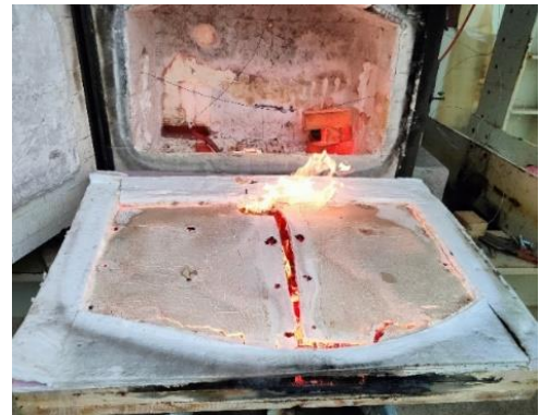
Figure 8. Gypsum Fireline plasterboard is intact with the specimen W-15FPJ
