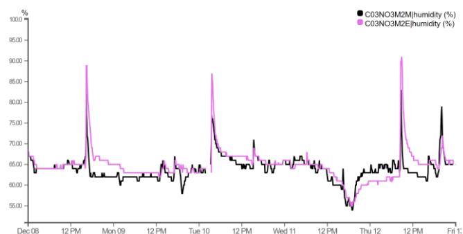
Figure 2: Typical RH data from a main bedroom (black) and ensuite bathroom (red) showing background values and peaks during showers.
