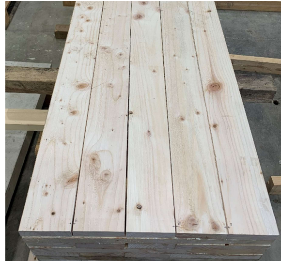
Figure 1. CLT panels made within the laboratory which showed gaps between lamella over time
