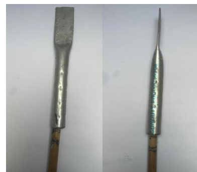
Figure 2: Steel tubes and epoxy used to provide grip on the bamboo culms in the pull-out tests
