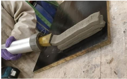
Figure 5. Printing with the specially developed nozzle and battery-operated aluminium gun
