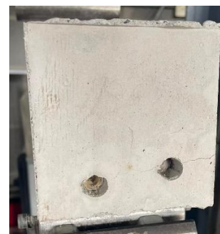
Figure 3. Bamboo bond failure during flexural test.
