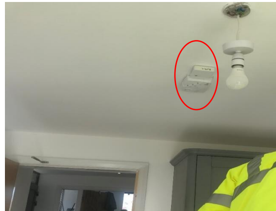
Figure 1. Ceiling mounted LoraWAN sensors.
