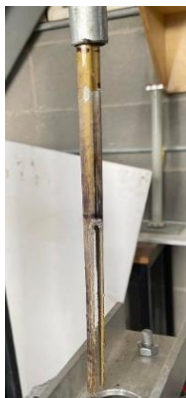
Figure 7: Embedded end displaying shear failure of culm under notch
