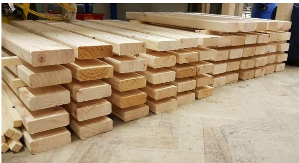
Figure 3. Arrangement of C16 timber samples drying in ambient conditions
