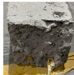
Figure 2. Bamboo tensile failure during flexural test.
