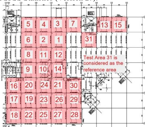
Figure 3: Individual slab locations in the floor during the assessment of composite metal deck slabs using the IR test.
