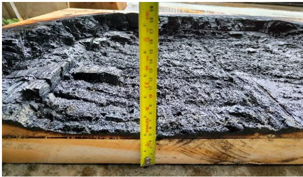
Figure 10. Measurement of uncharred depth
