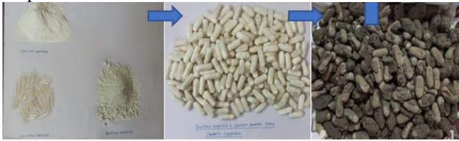
Fig. 5 Cement paste-coated gelatine capsules encapsulating bacteria.
