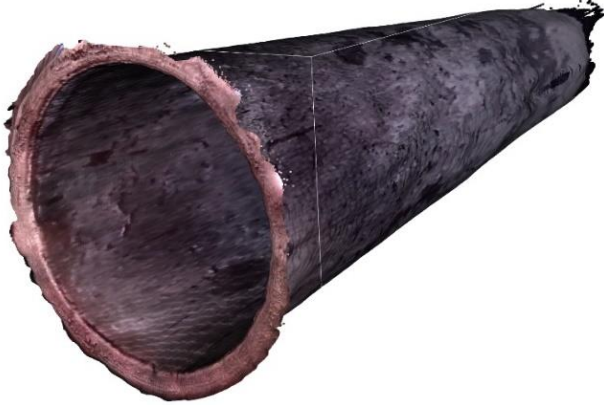
Figure 3. Point cloud of the spigot and interior of a Ø525 full-length drainage pipe as viewed from the spigot-end of the pipe. The socket (far) end of the pipe is poorly defined as much of the socket is occluded from the camera viewpoint.
