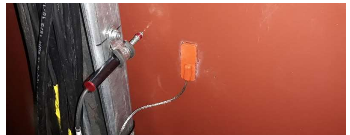
Figure 6. Displacement potentiometer and PT100 temperature sensor
