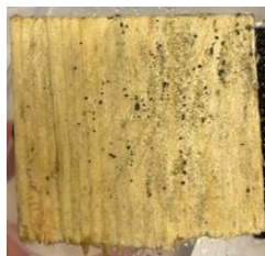
Figure 6. Untreated timber at 100% RH, 25°C in week 5.
