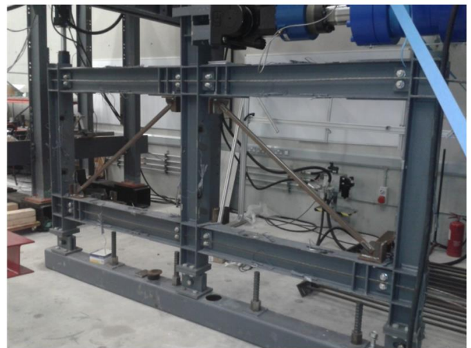
Figure 3. SC-CBF was designed for pushover testing (adapted from O'Reilly and Goggins [21]).
