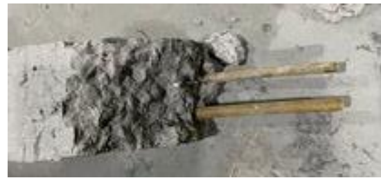
Figure 8: Half of an unnotched reinforced beam displaying bond failure along the culm
