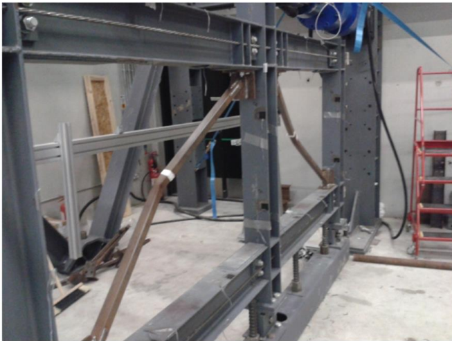
Figure 6. Deformation of the bracing members after testing (B4B specimens)
