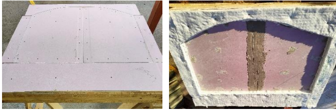
Figure 3. CLT panel protected with 15mm Fireline plasterboard with a vertical joint and a joint around the perimeter (W-15FPJ), Left: Joints are visible, Right: Joints are sealed and the panel is ready to be placed in the kiln for test
