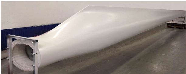
Figure 2 13 metre commercial wind turbine blade manufactured using an out of autoclave one shot process [1].
