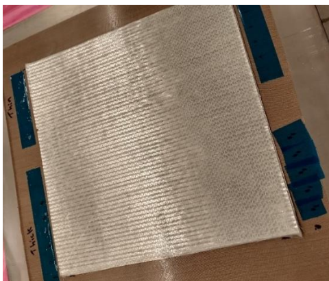
Figure 5. Glass Fibre Ply with Fibre Optic Cables Held by Heat-Resistant Tape
