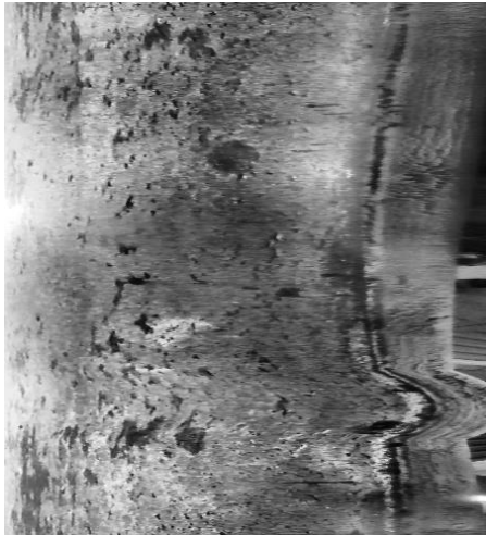
Figure 2. Linear Polar transformation of the interior pixels of a full-length drainage pipe. The far end of the pipe is to the left and the near end, including the spigot, is to the right.
