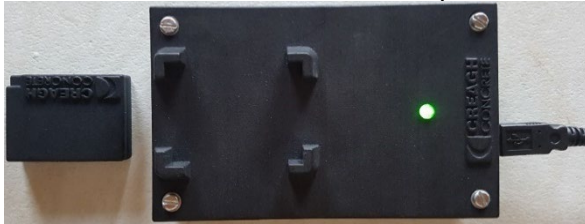
Figure 3 A typical sensor and the electronic module used for giving a unique ID.
