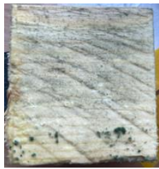
Figure 5. Untreated timber at 100% RH, 15°C in week 5.
