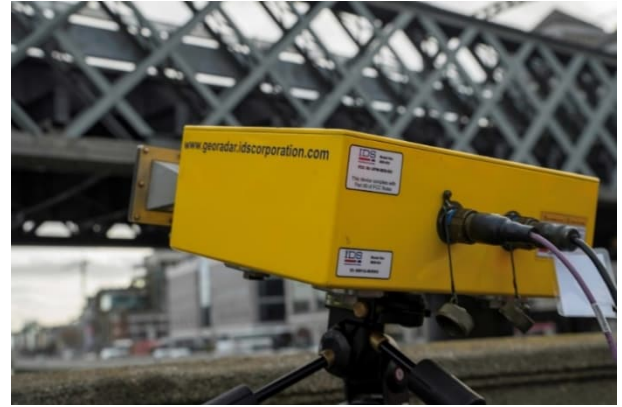
Figure 3. Interferometric radar set up at the Loopline Bridge.
