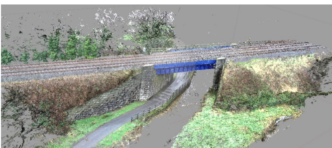
Figure 2. Newry Canal Dense Point Cloud – Photogrammetry Model
