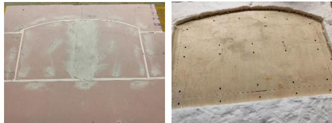
Figure 4. W-12.5FP25PW: 12.5mm gypsum fireline plasterboard placed between the CLT panel and the outer plywood layer (Left), Exposed 25mm plywood layer (Right)
