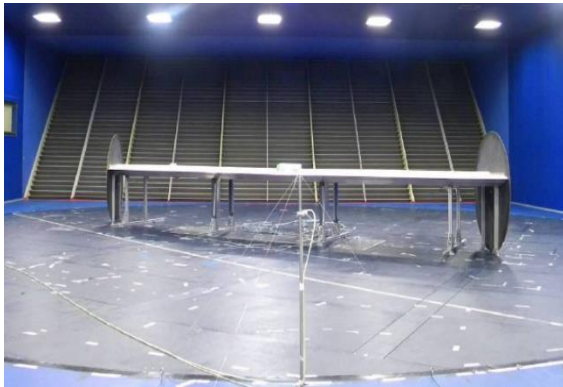
Figure 2. View of the bridge model in the wind tunnel [14]
