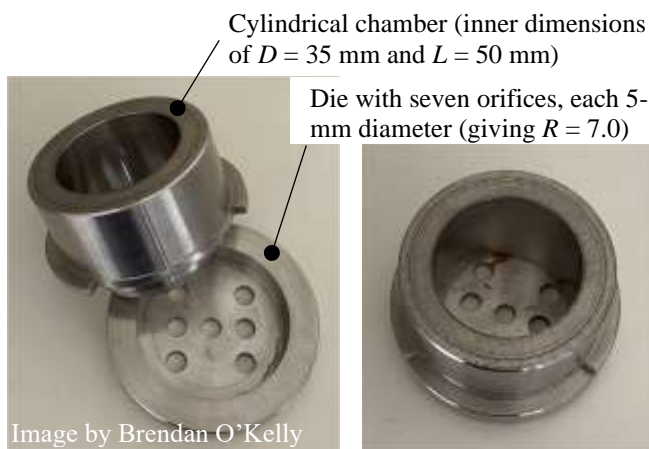
Figure 4. Chamber and die combination for LL testing in TCD extrusion apparatus: disassembled (left); assembled (right).
