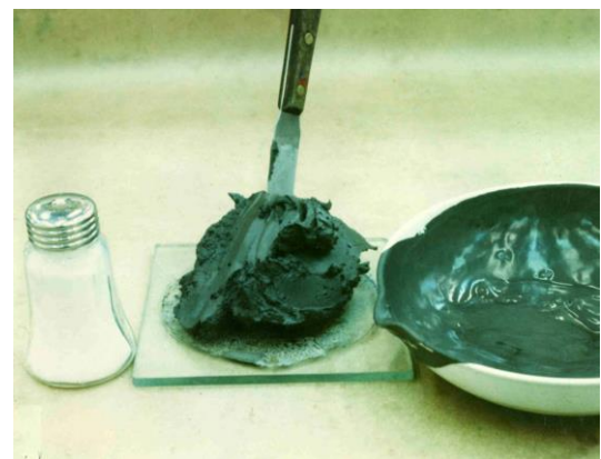
Figure 14. Adding salt can restore strength of disturbed quick clay. Image courtesy Kjell Karlsrud, NGI
